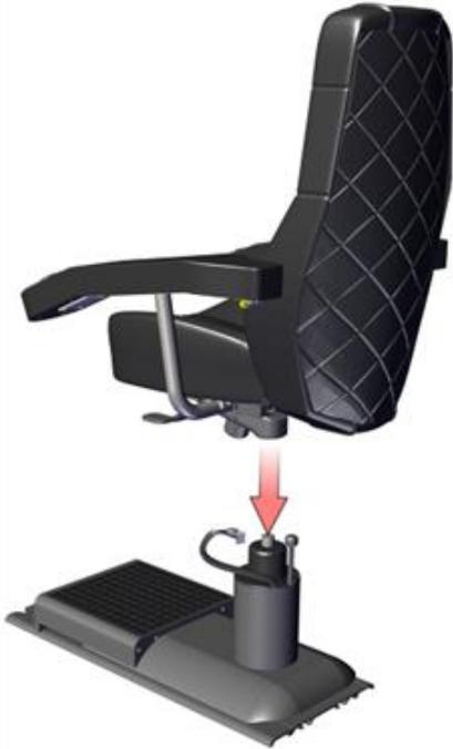
3. Plug in the connectors between the base and the top of the chair: remove the cover, plug in the connectors, switch on the earth wire connectors and then install the chair protective cover.
