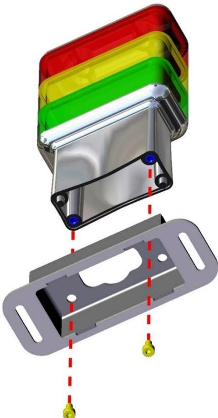
3. Mount the G50-50C-VIP.02.05.00.00.00.00.00 "Distance top lamp" part by 2 pcs. DIN 7985 M4x10 screw.
